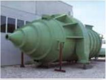
**mechanical pumps**, before them and after the stationary tank, a **Vacuum Bag Filter** is an essential equipment to assure a higher reliability of the vacuum pumps.
